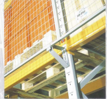
4 Safety mesh cladding - often used where a walkway is near stored pallets
