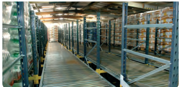
Ideal for perishable and time sensitive products pallet live storage saves space of up to 60% compared to conventional racking.
