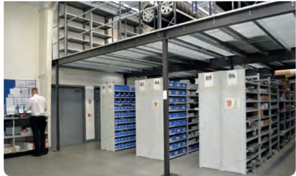
Extra space can be created by adding a mezzanine floor into the storage design, delivering extra floor space.
