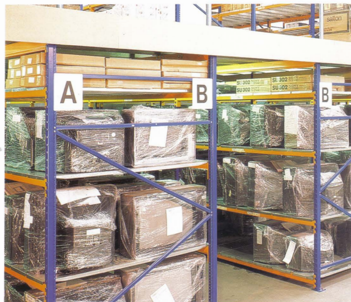
A typical two-tier shelving installation for the storage of electrical appliances.
