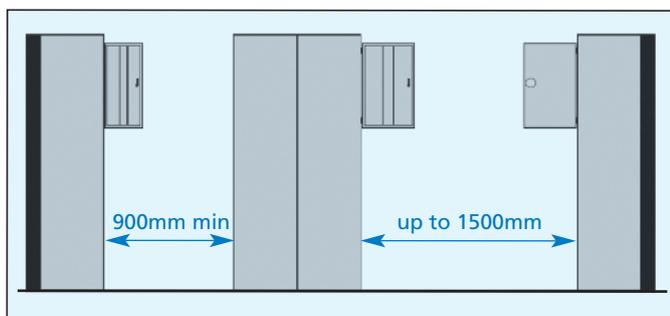
Lockers standing on support frames fitted with a seat should have a minimum aisle width of 900-1000mm between seats, but a spacing of 1200mm is desirable if facing lockers are to be used simultaneously.
